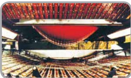
thermoforming of boat hulls
