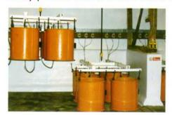
capacity of an oven. For example, one particular award winning installation of 3 THERMOSAFE units heats 20 drums per day. The ease at which capacity can be adjusted, to meet varying throughput demands and the varying heating requirements of different materials, is in stark contrast to the fixed facility of an oven.
