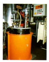
Uniform heating and instant response makes the heater ideal for removing residues from drums, significantly reducing wastage. With full drums, these same features enable very rapid removal of solid drum contents by melting the outer layer of material.
