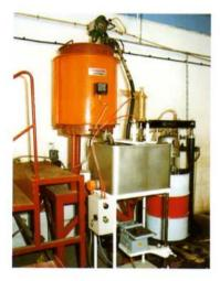
Complete access to the drum while heating enables pumps and stirrers to be employed. The drum and heater can be integrated into the system, often eliminating the first process vessel, and continuous feeding of material, at regulated temperature and flow rate, can easily be achieved.
