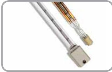
Halogen Infrared heaters emit in the near-infrared region and excel with very high radiation intensity and very fast response time. They are ideally suited for drying and curing processes where deep penetration and rapid response is required. They can be supplied with different reflective coatings and terminations.
