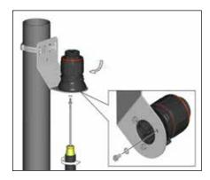
2. Mount expediter to bracket using M5 x 8mm screws and M5 lock washers. Tighten cap securely.
