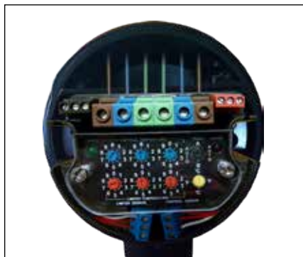
14. Install electronic control module and complete system wiring. Terminal set screws shall be tightened to a torque value of 1,4 Nm (12,4 lb-in). See wiring details. Set modules electronic control and/or control limiter at desired setpoints.
