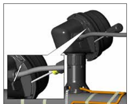
18. Lid latch mechanism fully engaged. To remove lid, repeat steps 16 and 17 but in the opposite direction.
