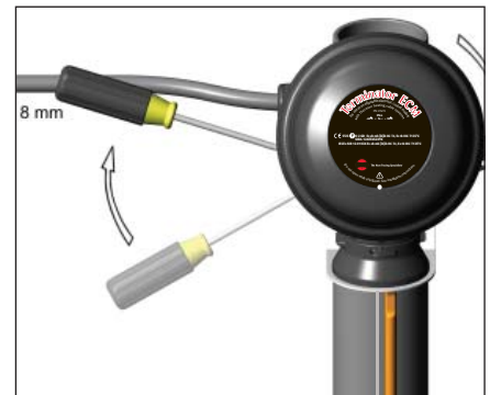
14. Use screwdriver to ratchet on junction box lid. Lid will rotate 30 degrees. To remove lid, repeat steps 13 and 14 but in the opposite direction.
