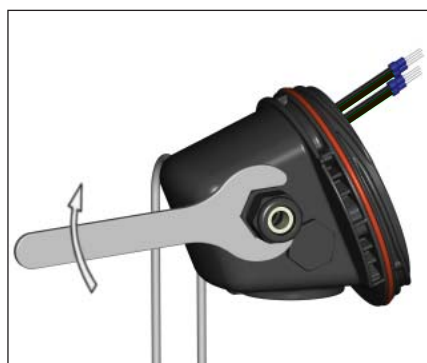
7. Remove M25 dust cap. Install M25 power gland (customer supplied) in M25 threaded entry.
